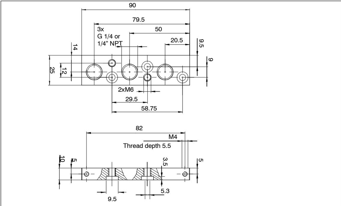
Figure 3-2 Dimensional drawing terminal strip for plastic housing
