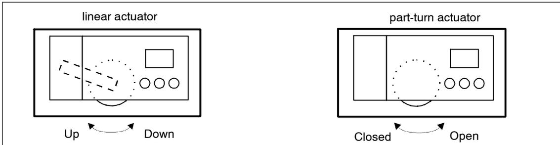
Figure 3-32 Direction of action of the actuators
