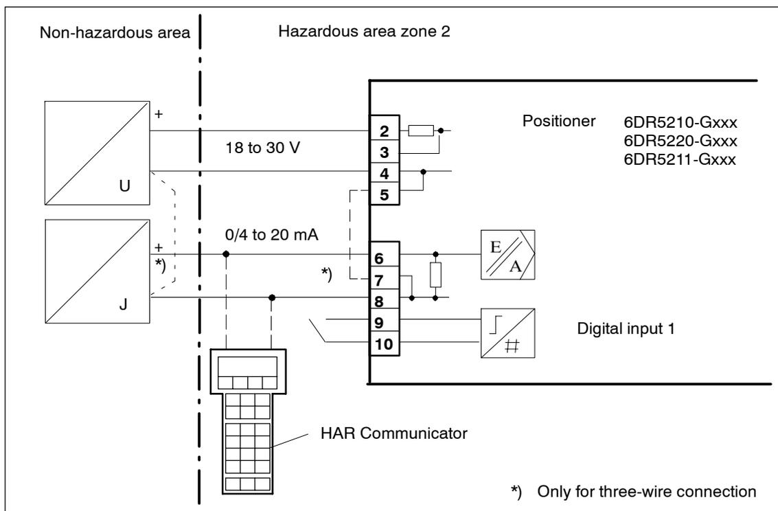
Figure 3-28 Three-/Four-wire connection, EEx n
