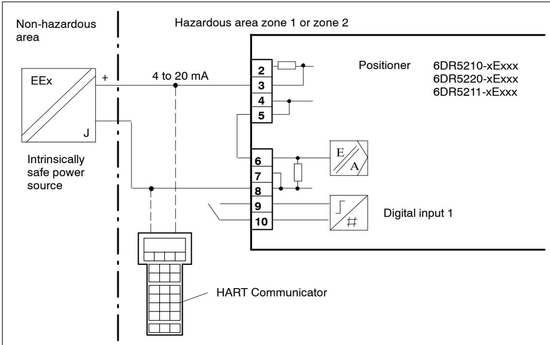
Figure 3-20 Two-wire connection, EEx i
