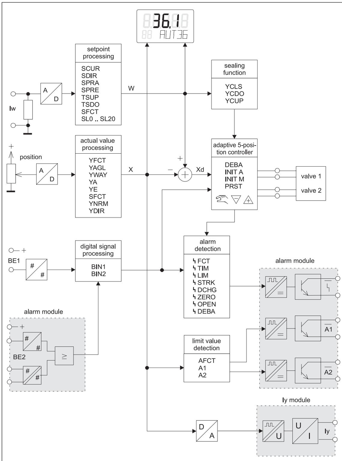
Figure 4-7 Configuration block diagram
