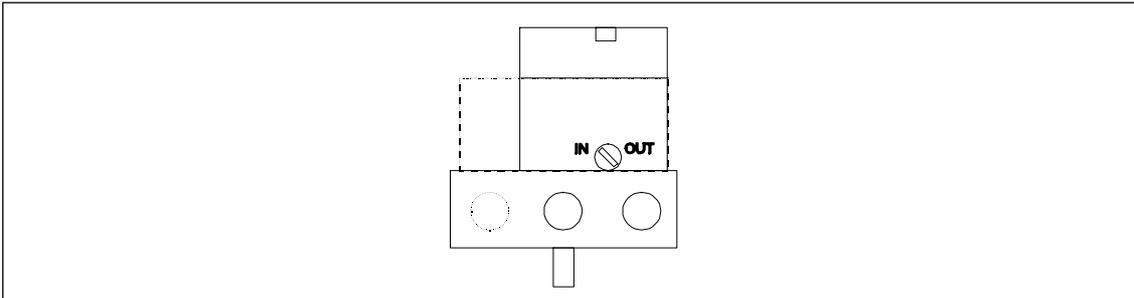
Figure 2-6 Purge air switch on the valve block, view of the positioner onto pneumatic connection side with cover open
