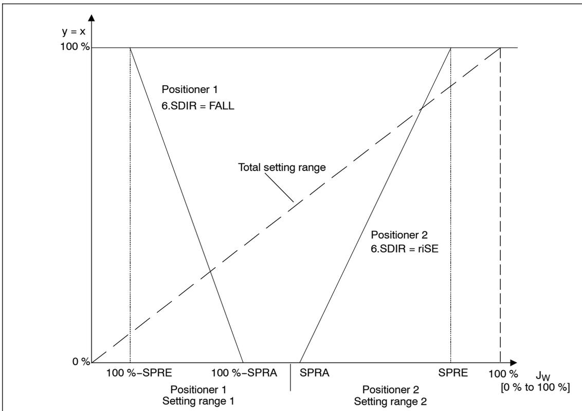
Figure 4-8 Example: Split range-operation with two positioners
