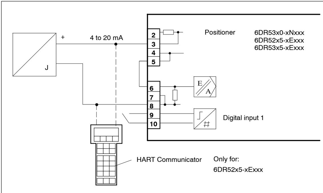
Figure 3-14 Two-wire connection
