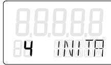
To exit the **Configuration** mode, press the operation mode key
