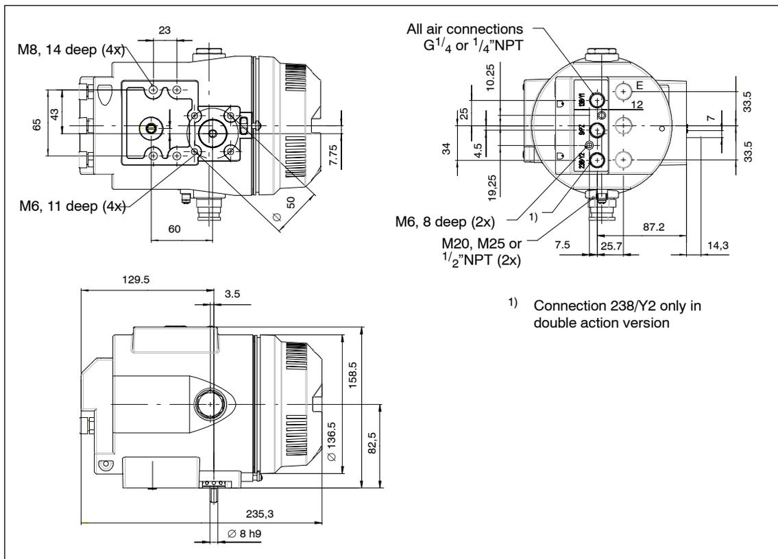
Figure 3-4 Dimensional drawing for positioner with metal housing in explosion proof version 6DR5x5
