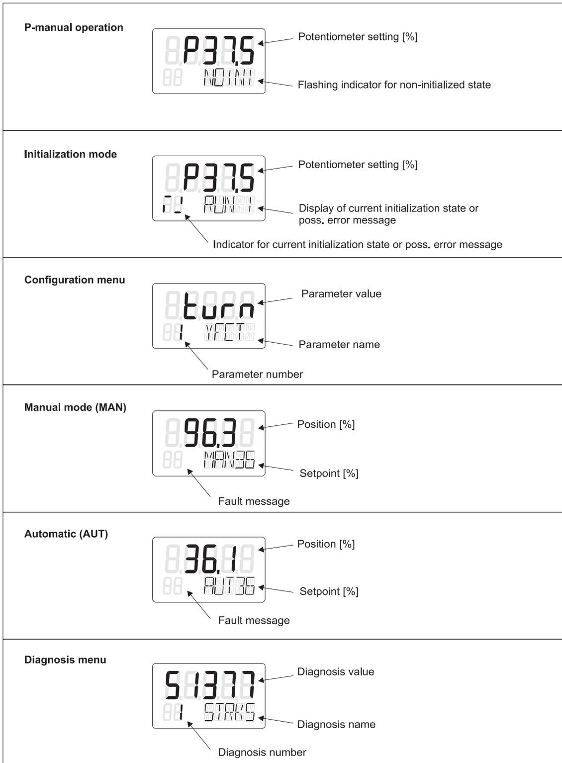
Figure 4-1 Meaning of the various display options
