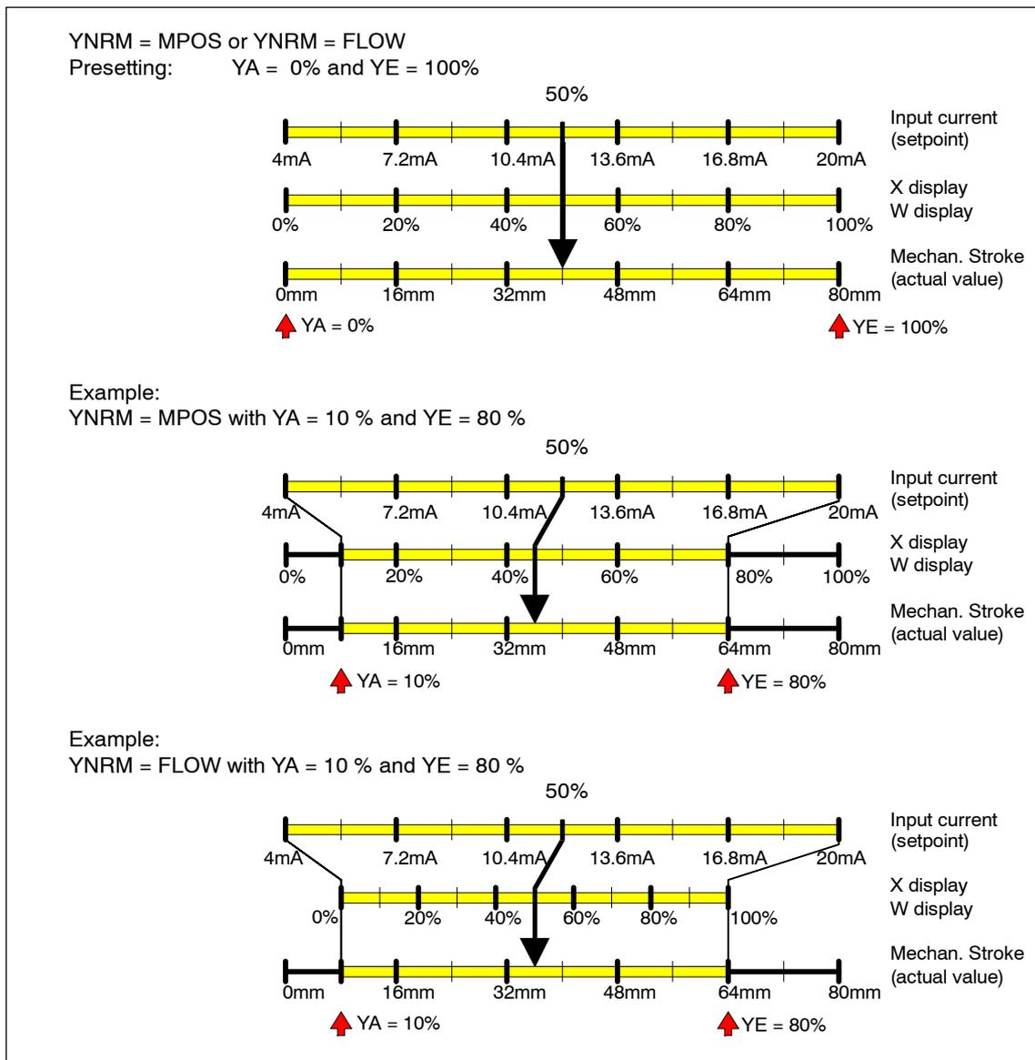
Figure 4-10 Dependence on the stroke of standardization and on YA and YE in the example of an 80 mm linear actuator
