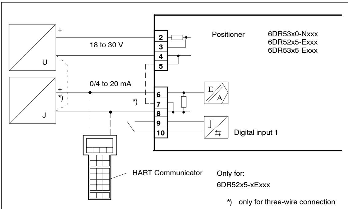
Figure 3-15 Three-/four-wire connection
